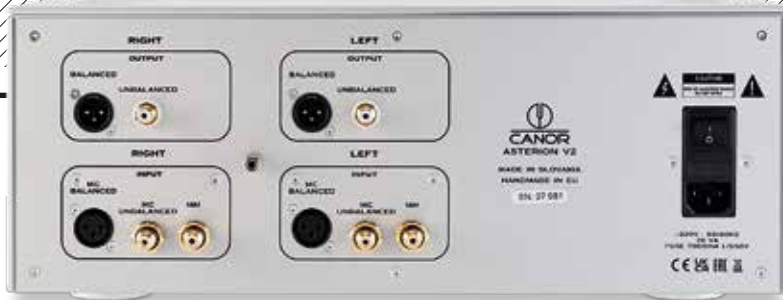
ABOVE: Standard single-ended RCA inputs are offered for one MM and one MC with an XLR for balanced MC connections. Outputs are on RCAs and balanced XLRs
